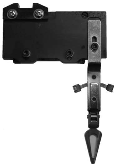
Fig.3-3-3 Yarn carrier for Lycra Tuck
